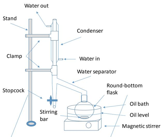
Picture 2. Water separator-assisted sulfonation of toluene in fume hood.
