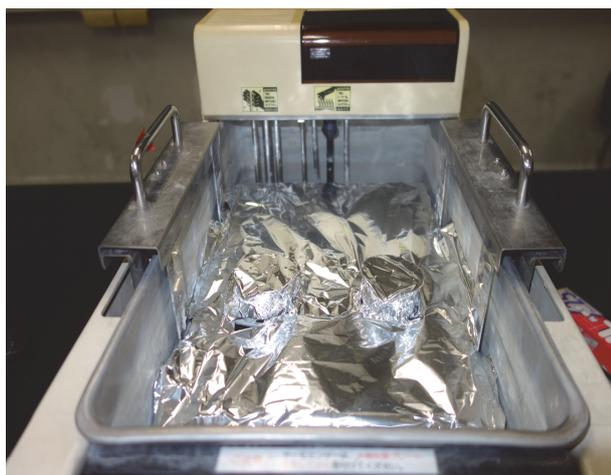
Picture 1. Shaker-assisted esterification. Beakers were covered with holed aluminum foil for releasing water vapor and preventing water from returning to the beakers.
